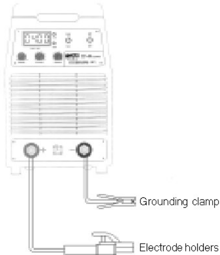
Equipping circuit configuration of arc welding (Picture8)
